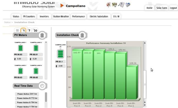
Once the inverter is detected you can enter the study of the series which feed that inverter as long as the plant has the string series monitored. This is done by clicking on the inverter marked
