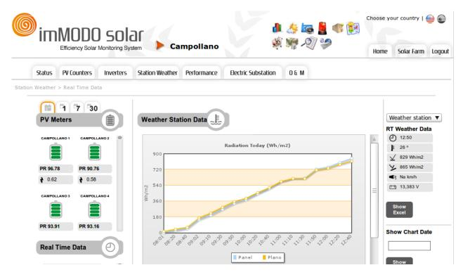
In the previous screen shot you can see a consultation of the radiation obtained by a plant by the flat sensor and the sensor inclined until 12:40, the time of the last data acquisition. If you scroll down this screen you can see other graphs fro temperature, wind, rainometer or any other sensor which the station has installed.
